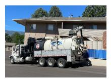
Building B Sewer repair continues as Colorado Springs Utilities has requested the HOA tag the Electrical & Gas lines. This required the HOA to utilize a HydroVac which would remove the water so the
